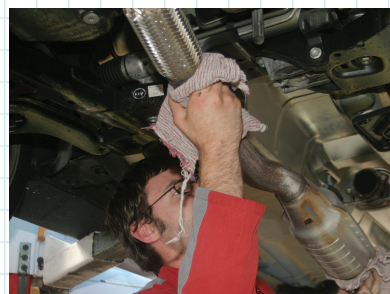
Turbo down pipe has to be replaced as part of the upgrade; penetrating oil is sprayed on (far left) as the retaining bolts for the down pipe have been known to shear off
