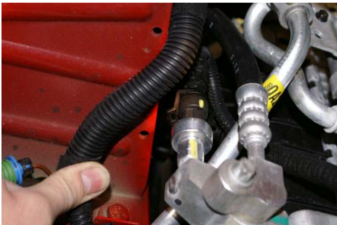
Picture 6 - Aircon Valve Clearance - Check.
