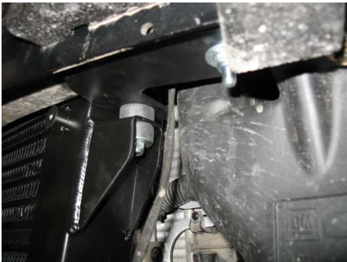
Picture 10 - Note positioning of rubber intercooler mounts.
