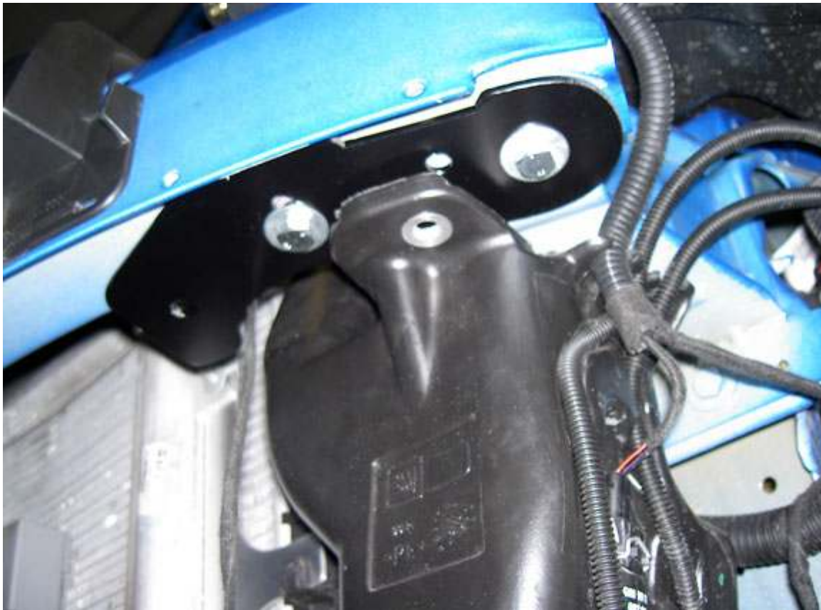
Picture 8 - Locating Bracket. One Each Side.
