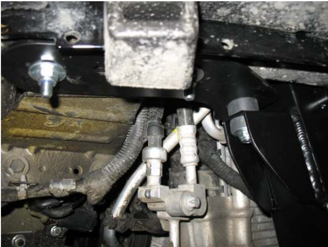
Picture 9 - Locating Bracket. One Each Side. Note bolt orientation
