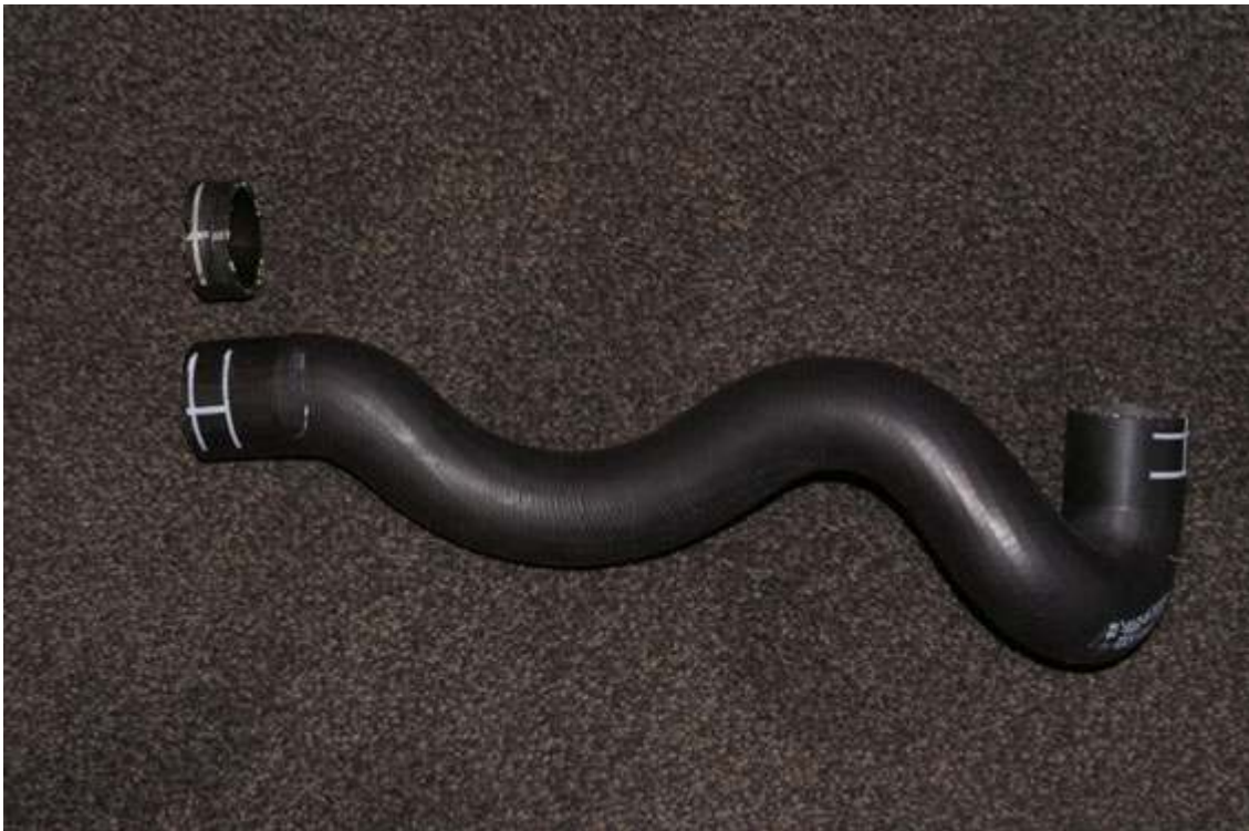
Picture 1 - Cut this small amount (shown top) from the end of the coolant inlet pipe onto the radiator.
