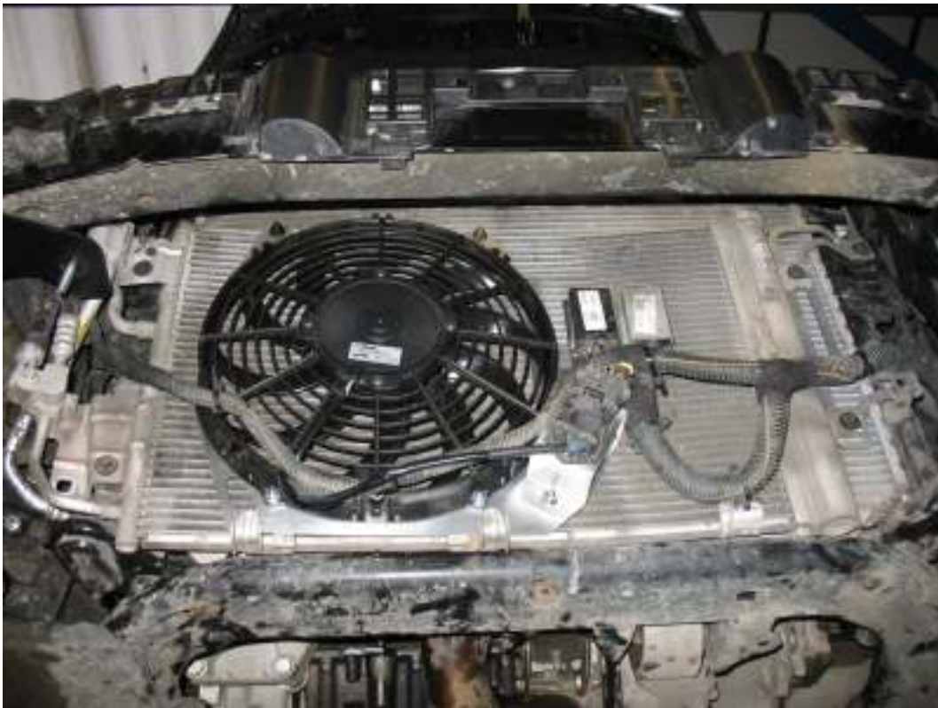
Picture 7 – Fan located on new bracket onto A/C condenser.
