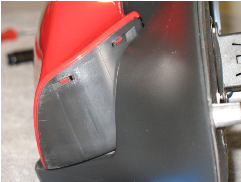
Picture of inner clips with mirror retracted back
