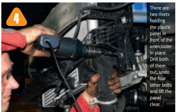
**4** There are two rivets holding the plastic panel in front of the intercooler in place. Drill both of them out, undo the four other bolts and lift the panel clear.
