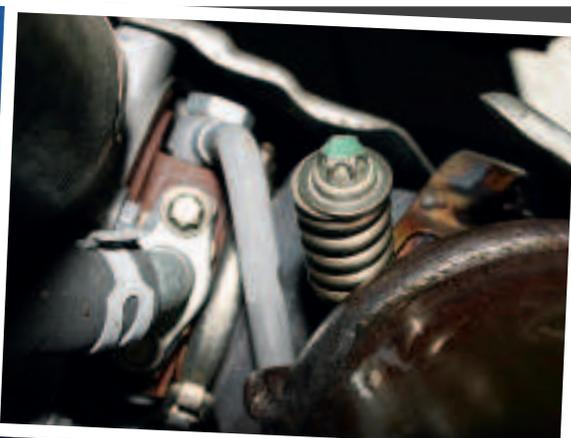
Moving to the front of the car, there is a spring clamp holding the catalyst to the manifold. It's hard to see, but easy enough to get a socket on the spring loaded bolt (the one with green paint). Slacken the clamp off and pull the catalyst clear.
