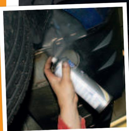
Lever the exhaust rubber from the bracket above the rear axle. Spraying the rubbers with lubricant first will make them easier to remove.
