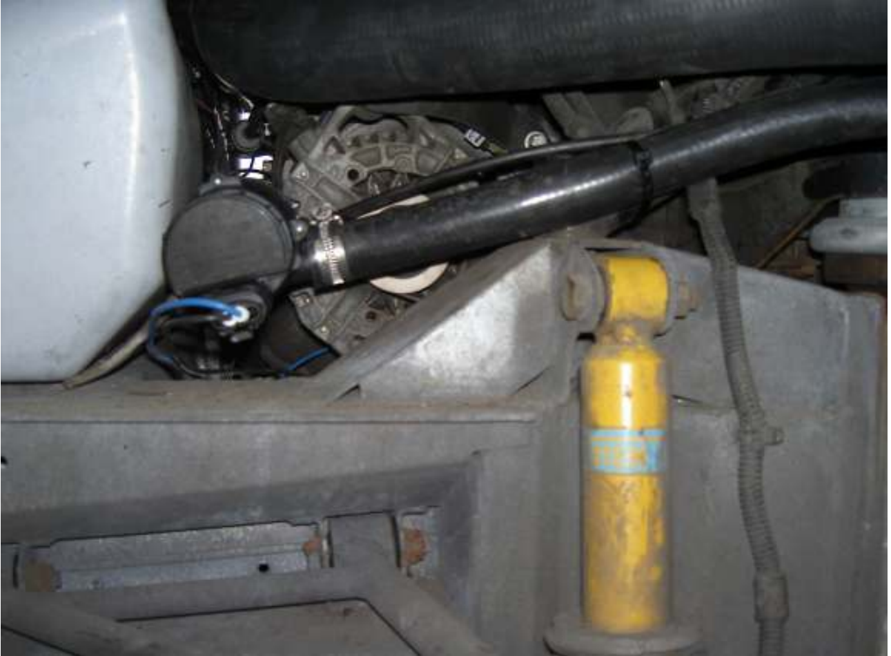
Pump Location – O/S/R behind wheel arch liner mounted on chassis:
