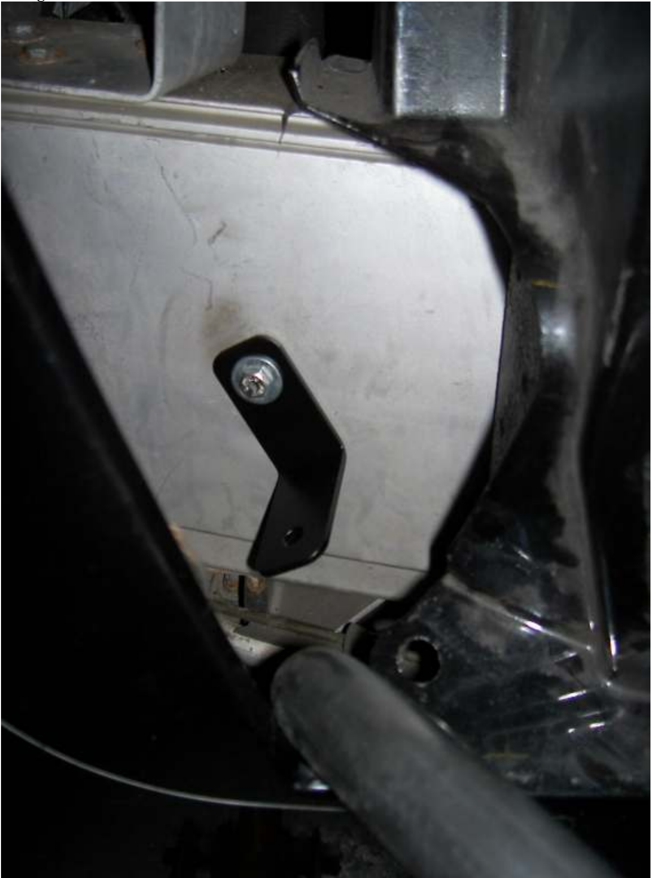
Charge Cooler Bottom Bracket:
