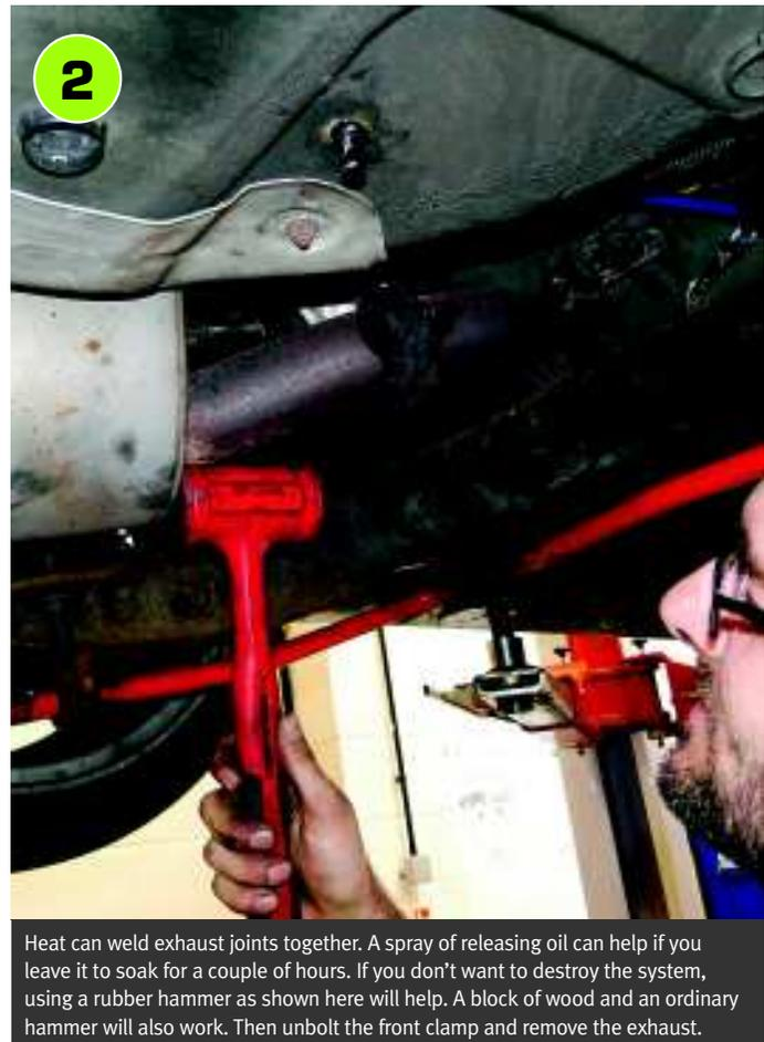
Heat can weld exhaust joints together. A spray of releasing oil can help if you leave it to soak for a couple of hours. If you don't want to destroy the system, using a rubber hammer as shown here will help. A block of wood and an ordinary hammer will also work. Then unbolt the front clamp and remove the exhaust.
