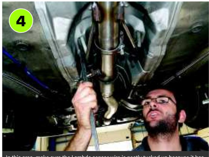
In this area, make sure the Lambda sensor wire is neatly tucked up because it has a habit of hanging a bit low. If necessary, careful levering on the appropriate body hanger bracket will bring the system into the central space to prevent contact with the body. Nobody likes an exhaust thumping off the floor!
