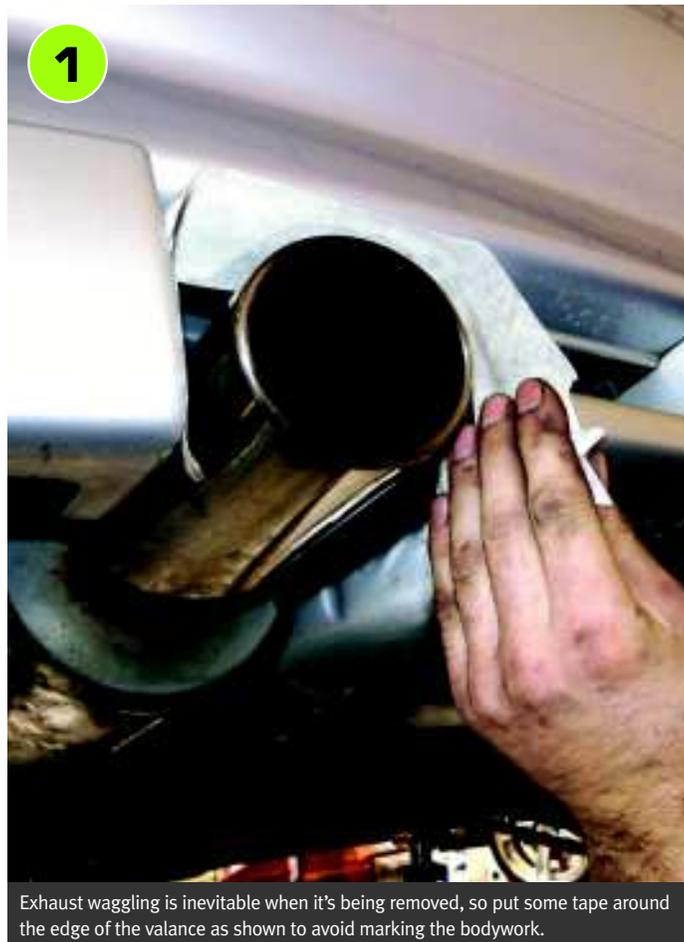
Exhaust waggling is inevitable when it's being removed, so put some tape around the edge of the valance as shown to avoid marking the bodywork.
