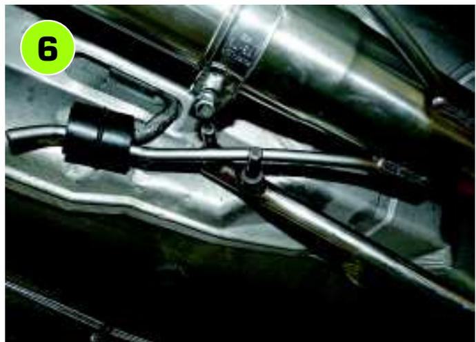
This shot shows a cam pulley tool - ideal for levering the exhaust mounting vertically. A large, open-ended spanner and grips could do the same thing, lowering or raising the height of the exhaust by cranking it up or down.
