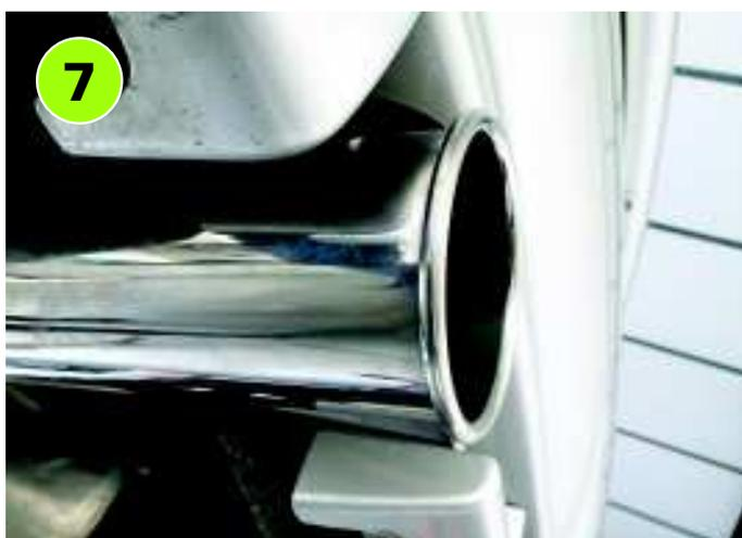
Getting near the end here, the owner was keen to avoid a boy racer look by having it nearly flush with the body. Alignment is achieved by carefully tapping the silencer with a rubber mallet. The silencer often has to be tensioned in the right direction as the clip is tightened in order to centre it.
