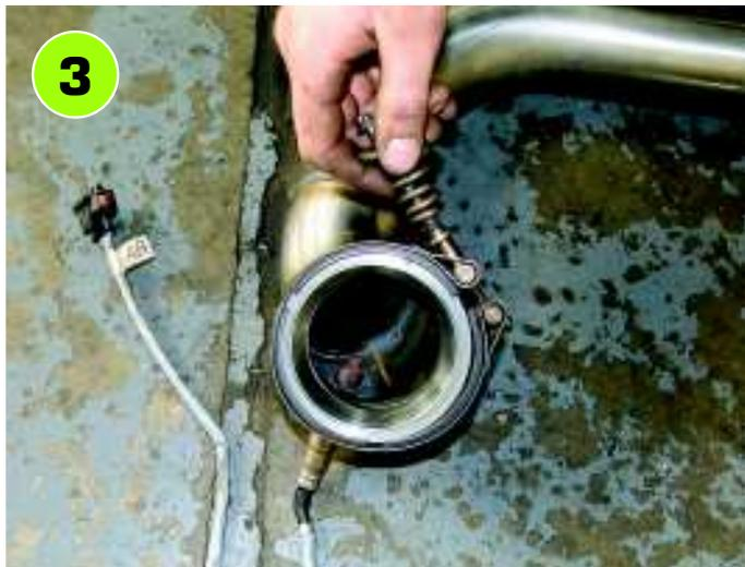
The main clamp bolt head needs to be easily accessible, but check that it's not likely to bash into anything with a bit of engine movement. Offer the downpipe up, tighten the clamp bolt up and the spring will do the rest.
