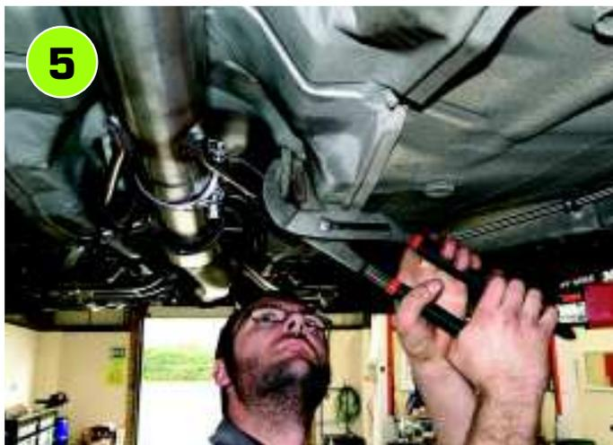
You'll ideally need large grips rather than a lever to pull the body-mounted exhaust hanger bracket away from the exhaust pipe. You may need to move brackets about on either side to achieve a fairly even tension on the rubber hangers.
