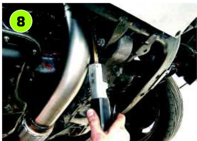
Here, a power hacksaw is used to remove about a centimetre off the corner of the front engine-mounting bracket where it sometimes gets very close to the exhaust downpipe, particularly on overrun. The gap can vary and some cars don't need it.
