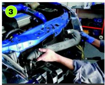
The improved direction of flow through the VXRacing intercooler means that this standard interconnection pipe is no longer required.
