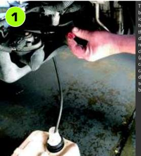
The grille/ bumper section ideally needs two people for the job to avoid damage during removal. Use a clean container (at least 4-litres capacity) to catch the drained coolant so that it can be re-used.
