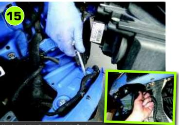
New longer bolts allow brackets to be fitted to support the new intercooler. The headlamps need to be moved aside first. A spacer inside the intercooler-to-bracket bolts means they can be tightened normally with no risk of crushing the rubber mounting bushes.
