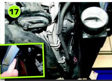
The lower mounting height of the replacement intercooler is so much more efficient - make sure that the fan and its wiring is not rubbing in this tight spot. The same goes for the boss on the front of the intercooler which must have a gap between it and the inside of the bumper support section.
