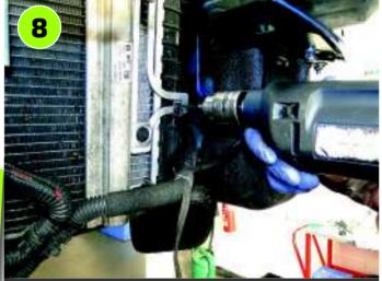
Extra security in retaining the bracket in the hook is achieved by using a 4 mm drill bit and a self-tapping screw. A piece of hacksaw blade can be pushed down behind the bracket to make sure the bit doesn't pierce the end of the radiator.
