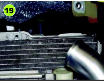
The larger bore pipe on its way to the intake goes across the top of the radiator which means a hacksaw and a file has to be taken to the U section. Make sure the pipe has no ragged edges where it's been cut.
