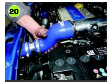
The hose might need a squirt of silicone lubricant as it has to be pushed a long way over the Courtenay MAP sensor pipe shown here, which had already been installed by the owner. The hose also fits over the original plastic pipe.
