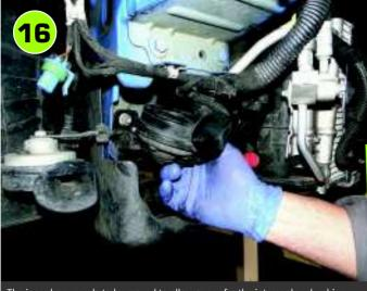
The inner horn needs to be moved to allow space for the intercooler plumbing. Unbolt the horn complete with bracket and mount it on the same bolt as the outer horn so that it sits just above it.
