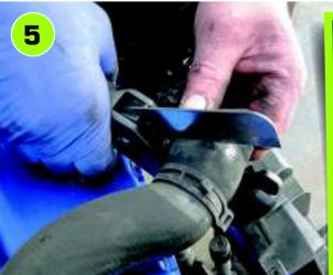
Courtenay technicians use a special tool - the easiest DIY way of cutting it square is to move the clip up to the point where it needs to be sliced and use it as a guide. A simple v-notch cut in the marked position provides the new index point for refitting.
