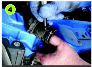
The radiator doesn't need to be removed but will be re-sited closer to the engine by about 25 mm. Cutting off the 'clean' part of the hose which was covered by the clip will shorten it by the correct amount. A marker pen is used to indicate where the small location notch needs to be cut once the hose has been shortened.
