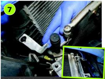
New brackets for the condenser come with the kit. Both brackets use existing captive nuts on the radiator, apart from the hook section holding the lower part of the right hand bracket.
