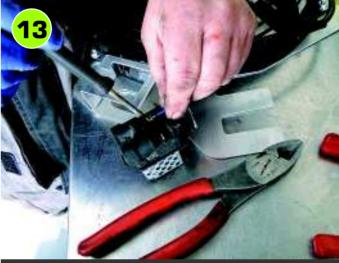
The new slimmer fan assembly has brackets to take the connector block and relays. The blue wire from the new fan is soldered on to where the red (positive) wire went.
