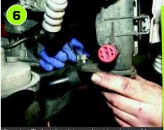
The next modification to the radiator mountings takes advantage of the Astra's reversible rubber mounting in the bracket being removed here. The mounting is easily prised out of its oval hole and turned 180 degrees to bring the radiator further back to make room for the new intercooler.
