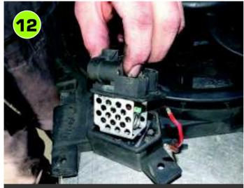
The original fan is too bulky to fit between the intercooler and the condenser but savings are made by robbing the connector/resistor block from the old one to fit to the new. De-solder the two wires and note where the red wire is attached.
