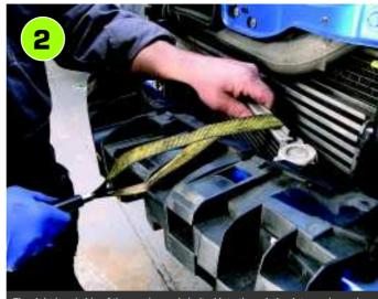
The right hand side of the condenser is bolted into the existing intercooler end housing. Once it's free, damage can be avoided by carefully strapping it out of the way during the strip-down.
