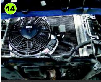
The fan adaptor plate allows the new fan assembly to bolt straight on to the original mounting points on the condenser.  $\frac{1}{2} \int_{\mathbb{R}^{n}} \frac{1}{2} \int_{\mathbb$
