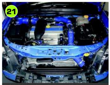
The finished job is so much neater than the standard plumbing. It's worth giving all the clips a small final tweak and everything a clearance check before refitting the front panel.
