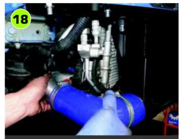
Larger bore pipe runs are a massive improvement over standard. Pressures in excess of 1.3 bar means that the worm drive clips need to be good and tight. It's worth making sure that everything is grease-free before assembly.
