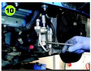
The original mounting bolt can be used through the new hole - bear in mind that the captive nut is mounted in plastic so care is needed not to over-tighten as it bites down on the curve of the bracket.
