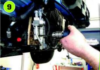
The original condenser mounting bracket is still used bottom left but needs to be drilled about 30 mm to the right as shown. A piece of wood behind the bracket is essential to avoid slip-ups. If it's not quite in line with the captive nut on the end of the radiator, it can be elongated using a round file.
