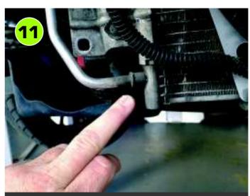
With the condenser in its new position, make sure that the tube (shown) clears the radiator and the valve plumbing is clear of bumper support. Touching in this area could eventually cause an expensive leak.
